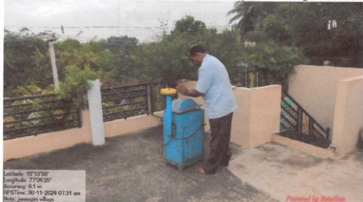
Photograph showing Continuous Air Quality Monitoring Station
